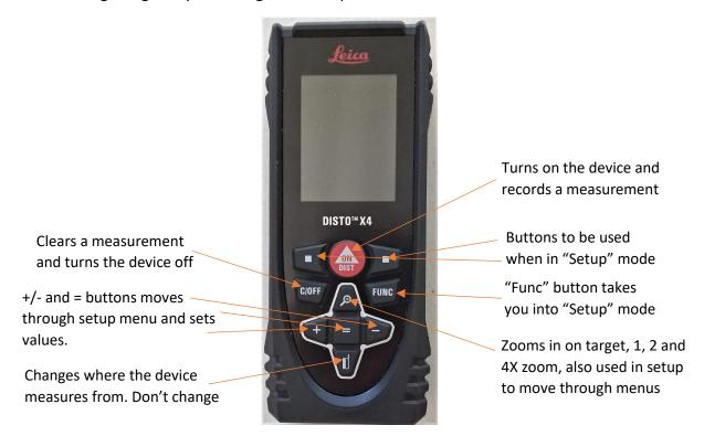
The offset is to be used when using the Measuring Stick. The amount of offset is the height of the stick plus the diameter of the crossbar. To determine the offset distance, lay the crossbar on the apron, butt one end of the measuring stick to the crossbar and measure the distance from the outside of the crossbar to the other end of the measuring stick. Let's say the measurement is 1.328m.
